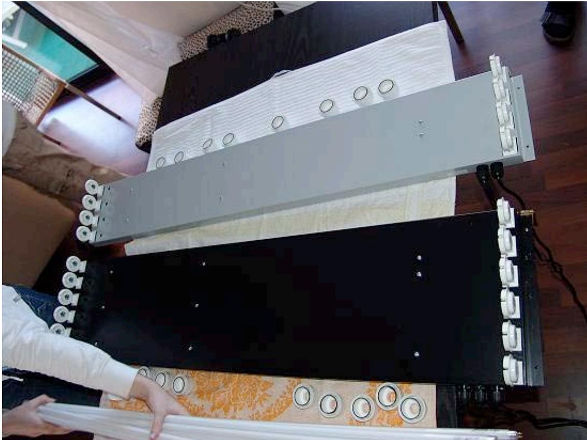
The lights above the tank are two blocks with ten 60" (80W) T5 tubes, so a total of 20 tubes (1600 W total lights) is installed.
